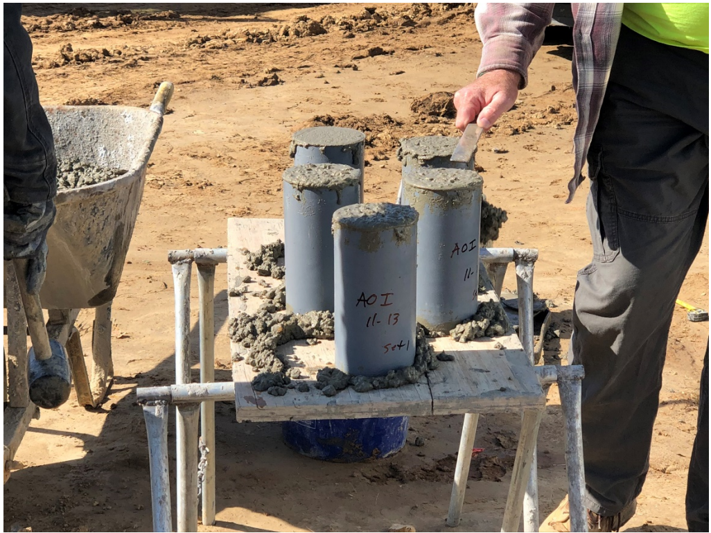
Figure 21 – Concrete Test Cores
