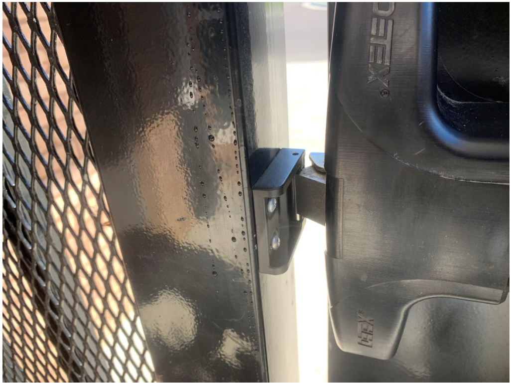
Figure 53 – Adjust Latch so Gate cannot be pulled open
