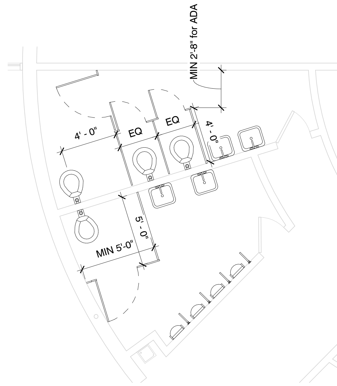
8 East Building North Toilets - New Const. Alt. #4 1/4" = 1'-0"
