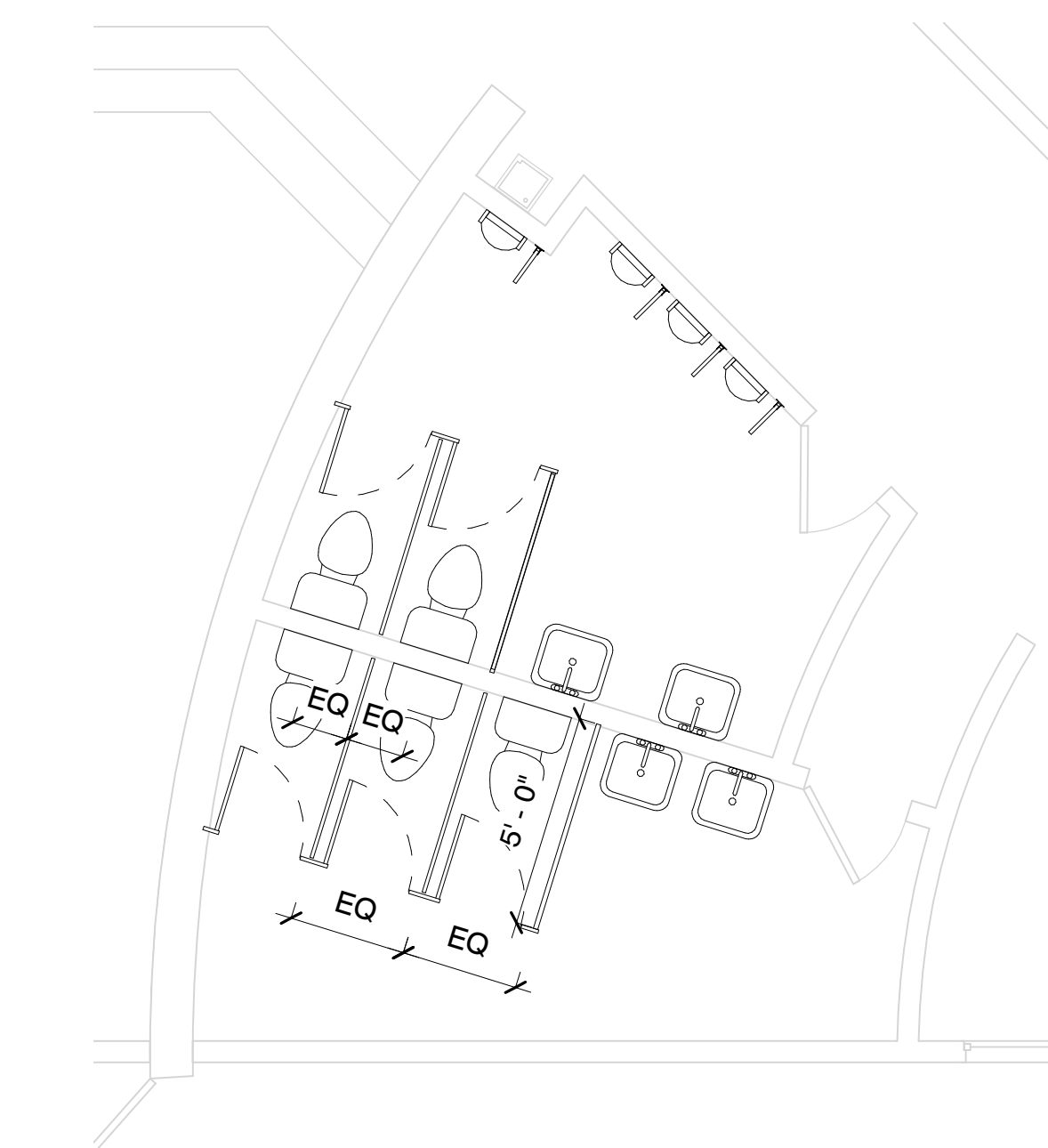
9 East Building South Toilets - New Const. Alt. #4 1/4" = 1'-0"
