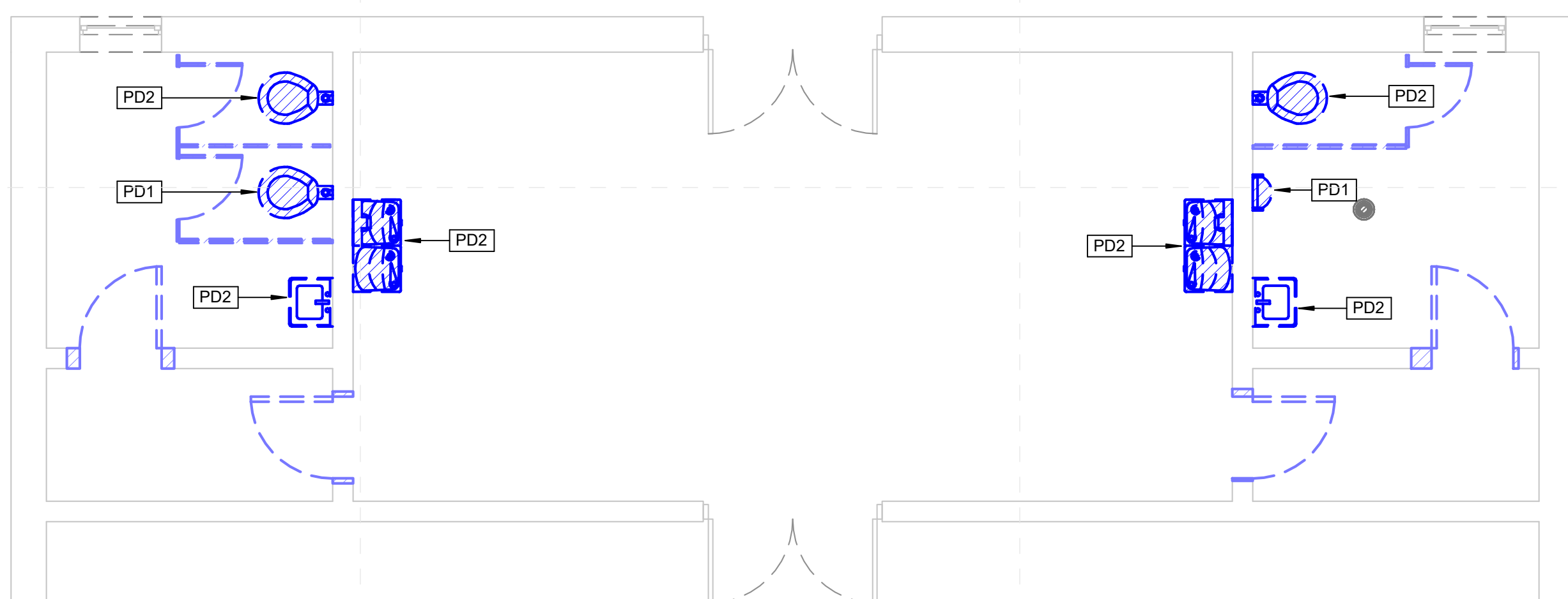
3 Lockard Elementary - Enlarged Plumbing Demo Plan (4) M-302d 1/4" = 1'-0"
